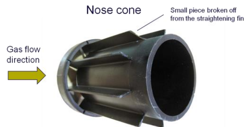
Figure 7 Laboratory tests showed that small damage on the nose cone resulted in a measurement error of nearly 2%
