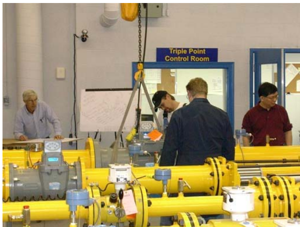
Figure 4: Testing Turbine Meters in CO 2 at Triple Point
