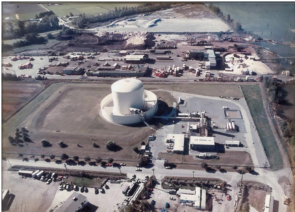
Photograph 1: Aerial view to southwest, 1995, of peakshaving facility with original storage tank, supporting infrastructure, surrounding concrete dam (white), and earthen berm. Area to west of the berm is still agricultural field, while the two properties to north are occupied by the sawmill, and piles of wood waste from the mill, respectively (image courtesy of FortisBC).
