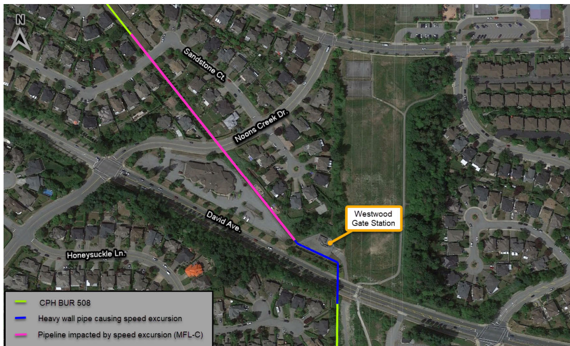
Figure 5: Example of a speed excursion resulting from a heavy wall segment on the CPH BUR 508 pipeline
