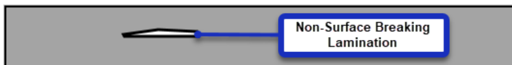
Figure 3 Example of a Non-Surface Breaking Lamination in a Steel Plate
