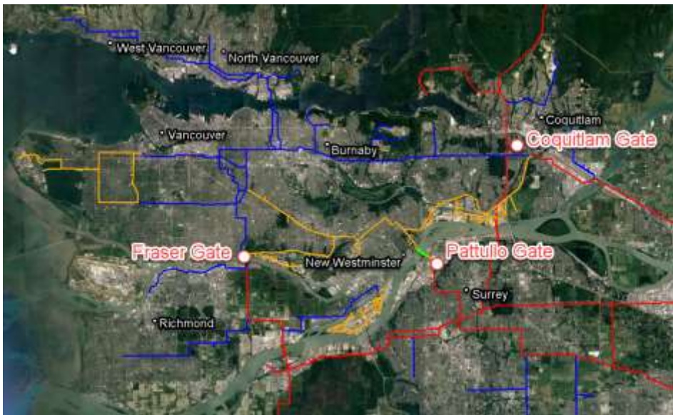
Figure 3-3: Gate Stations Feeding FEI's Metro Vancouver Distribution System
