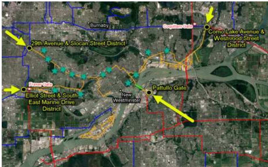
Figure 3-2: Stations Supplying the Metro Vancouver 700 kPa Trunk Distribution System
