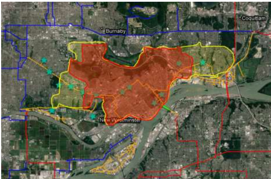
Figure 3-5: 25,500 Customers Impacted by Loss of Pattullo Gas Line Feed in 2039
