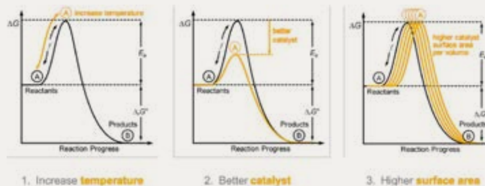
FIGURE 17: Impacts of different methods to improve kinetics of pyrolysis reaction 35
