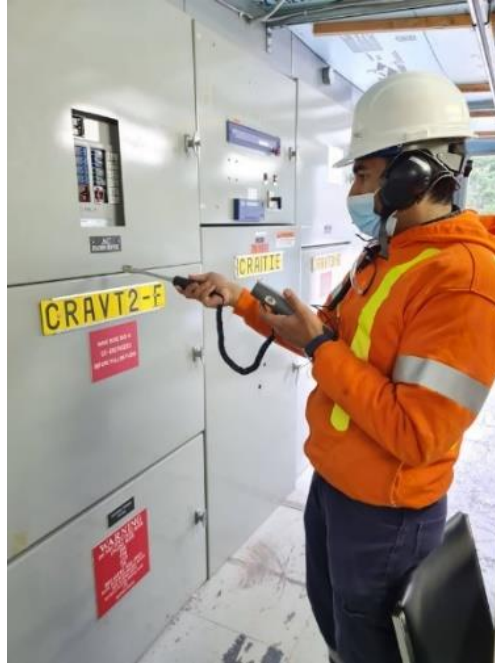
Figure 1: Online PD testing performed using a handheld PD measuring instrument
