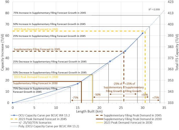
OCU Pipe Length vs Incremental Capacity
