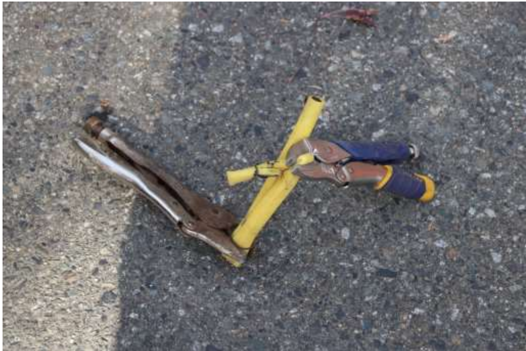
Photos 8 and 9: Makeshift Repair Attempts by Contractors In An Effort to Conceal Damage to Gas Lines
