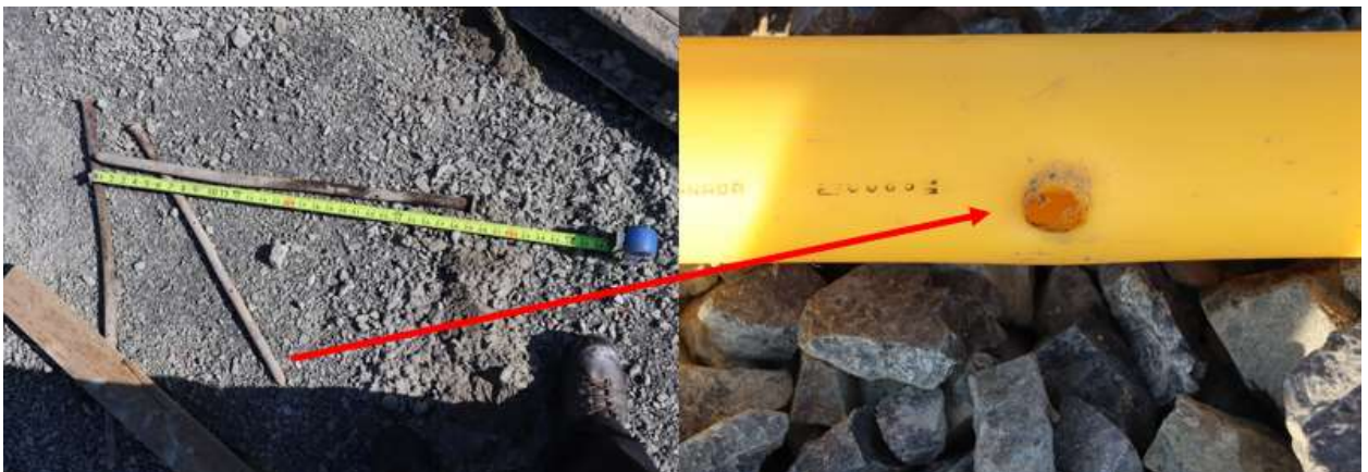
24 Photo 3: Service Line Puncture from Stake
