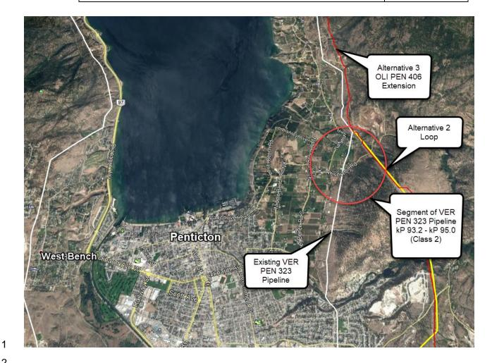
33.2.1 If Alternative 1 was implemented and the VER PEN 323 MOP was reestablished to 6619 kPa, confirm whether a class location change from 2 to 3 in this segment (kp 93.2 to 95) would cause the MOP to be derated. To what MOP would the pipeline be derated? How would this affect the ITS capacity?
