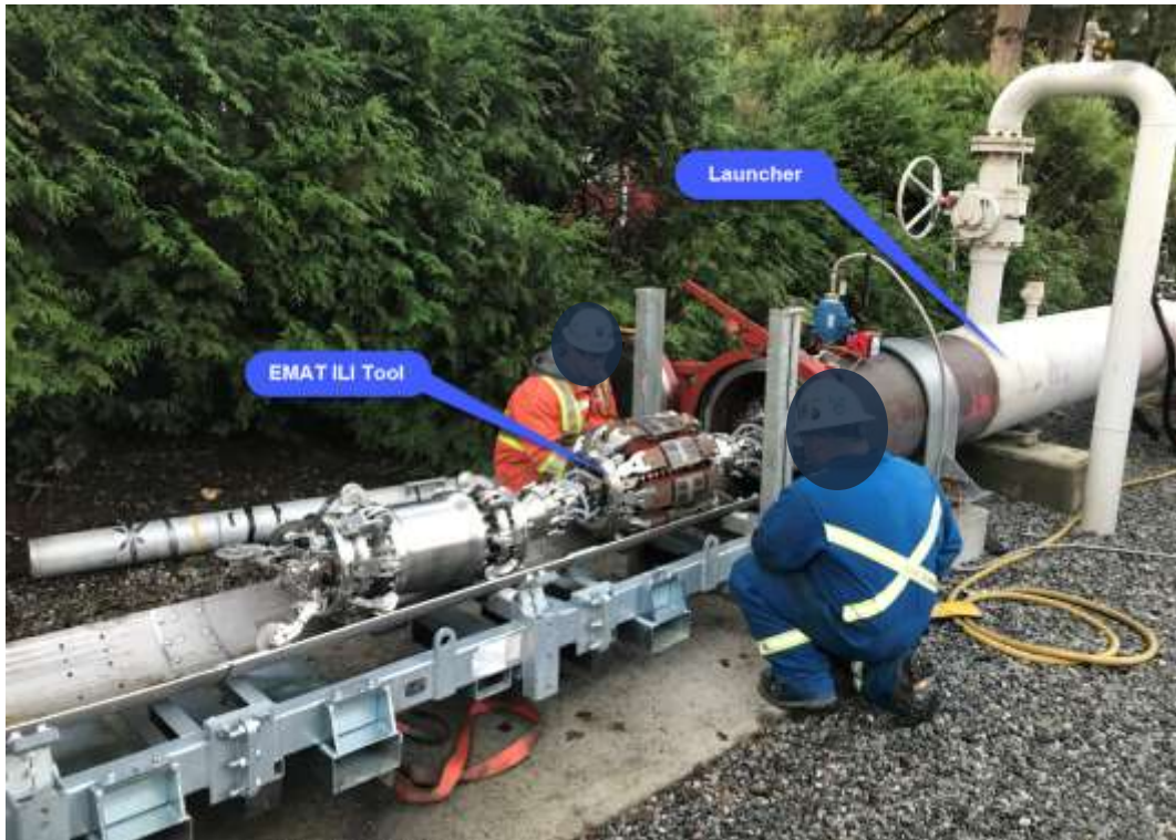
Figure 4-2: EMAT ILI Tool being Inserted into a Launcher
