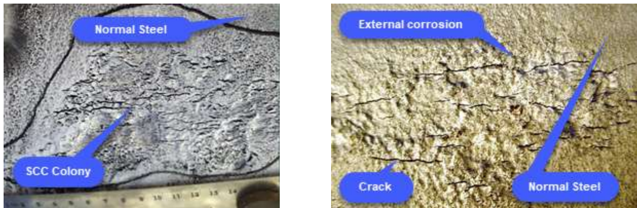
Figure 3-10: Examples of Stress Corrosion Cracking as Identified on FEI's Transmission Pipelines
