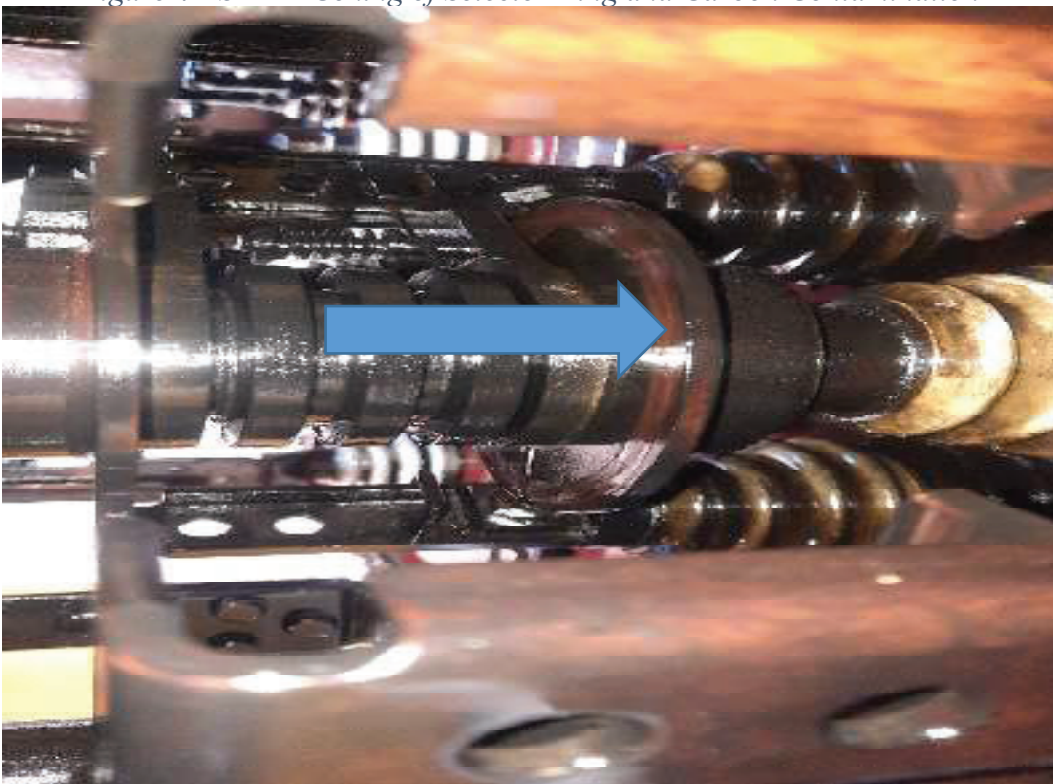
Figure 4 ASM T2 Coking of Selector Ring and Carbon Contamination
