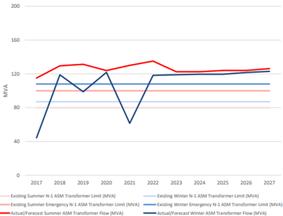
Figure 3-7: ASM Terminal Station's Contribution to the Boundary and Similkameen Areas' Total Load Compared to the N-1 Transformer Limits 13
