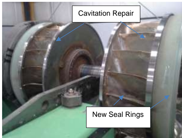
2 3 Figure B2-3: Turbine Refurbishment
