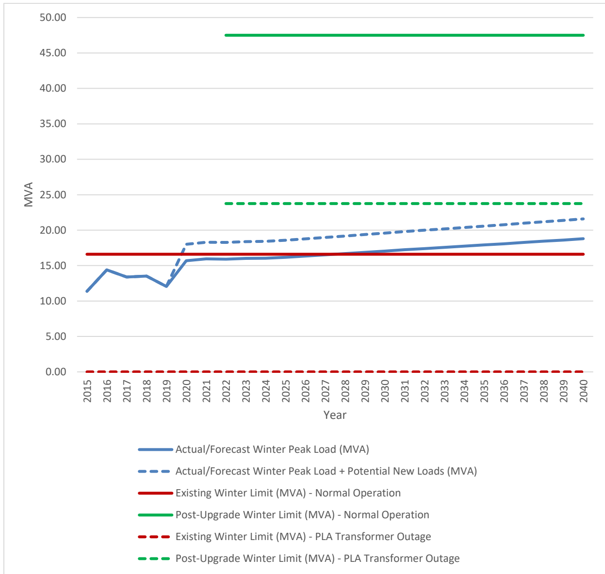
1 Figure 3: PLA Area Winter Peak Load and Limits Under Alternative A (2x20 MVA)
