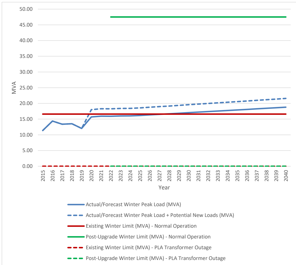
Figure 4: PLA Area Winter Peak Load and Limits Under Alternative B (1x40 MVA)
