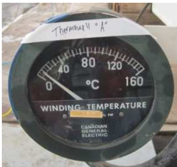
Figure 4: The Model FW temperature gauge contains a faulty contact used for fan control
